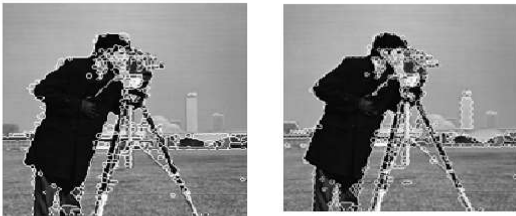
Fig 4: Clustered Cameraman image using Proposed Hybrid Clustering Algorithm with Clustering Radius and Threshold value 5
